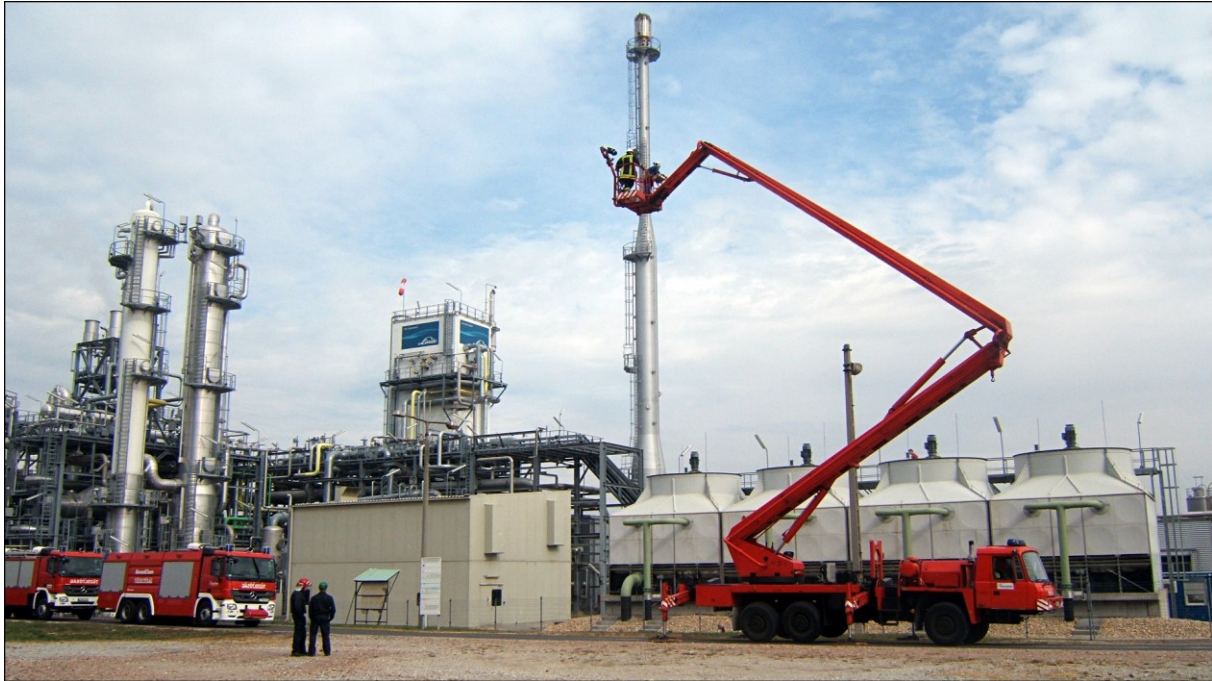
Figure 3 – Sound propagation measurements up in the air with the help of the fire department
